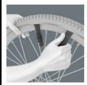
The 9503 tyre lever can be used as a valve ejector for Sclaverand (French) valves and as a bleeder valve for car valves.
