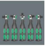
The ratchet head pivots freely and can be locked into any defined position by using the slide switch that is positioned on either side. It is even possible to work in very confined and difficult-to-access areas with enhanced hand clearance. The predefined locking at 0°, 15° and 90°, both to the right and
